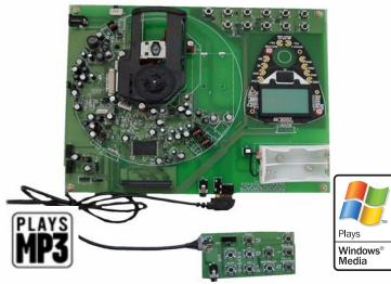
The CRD7410-BA is powered by the highly integrated Cirrus CS7410 solution for CD/MP3/WMA players. The CS7410 integrates microcontroller and DSP capability into a single device to provide a highly cost effective and compact solution for this exciting new class of consumer electronics products.
